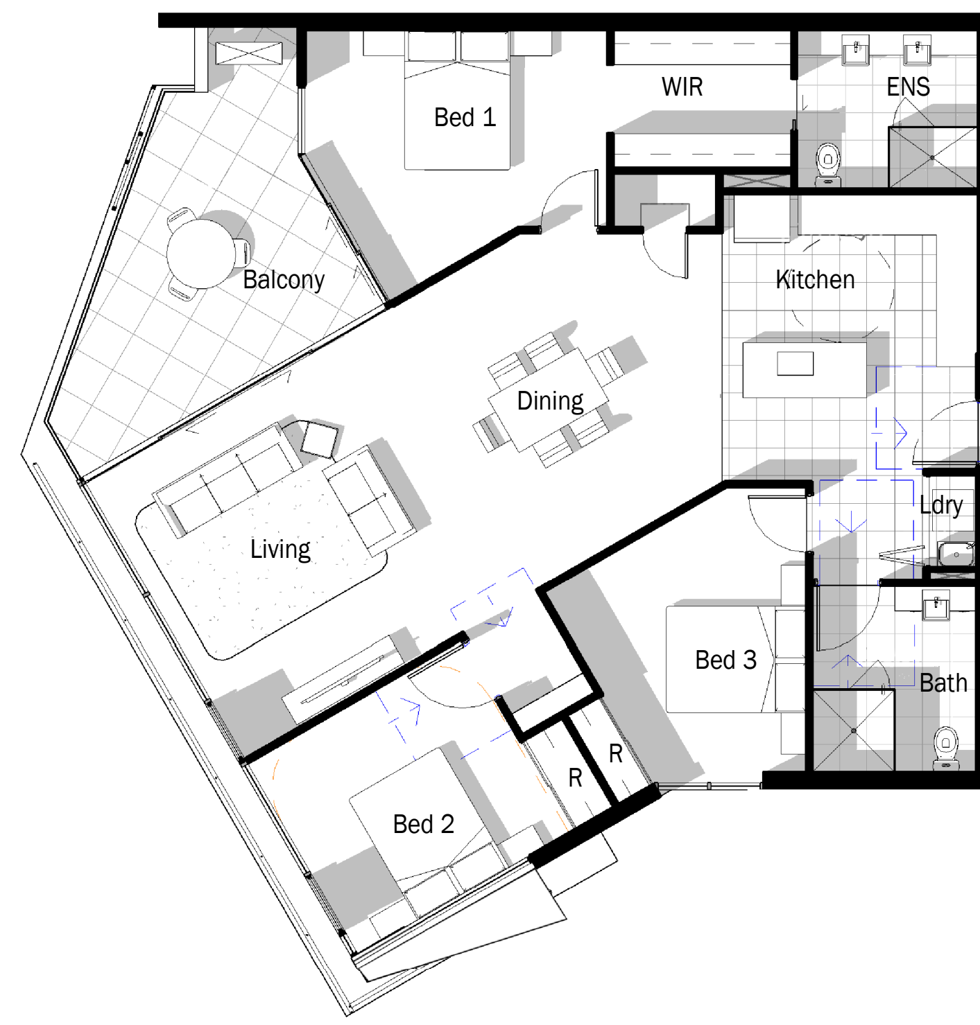
Typical Unit - (3A.1) layout for future compliance with AS4299
